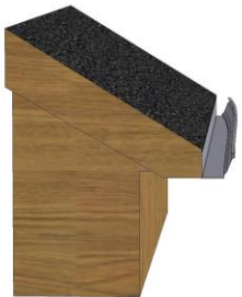
GUTTER LIP RUNNING INTO THE HOUSE
