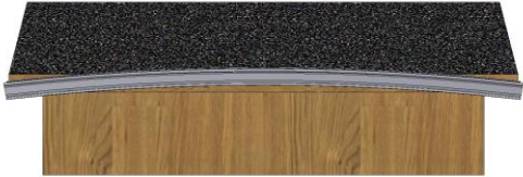
GUTTER RUNNING DOWNHILL
